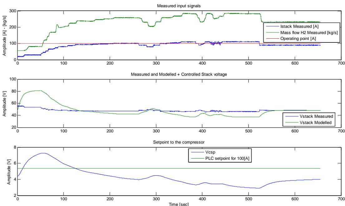
Figure 10. Controlled Stack Voltage and Compressor Set point.
