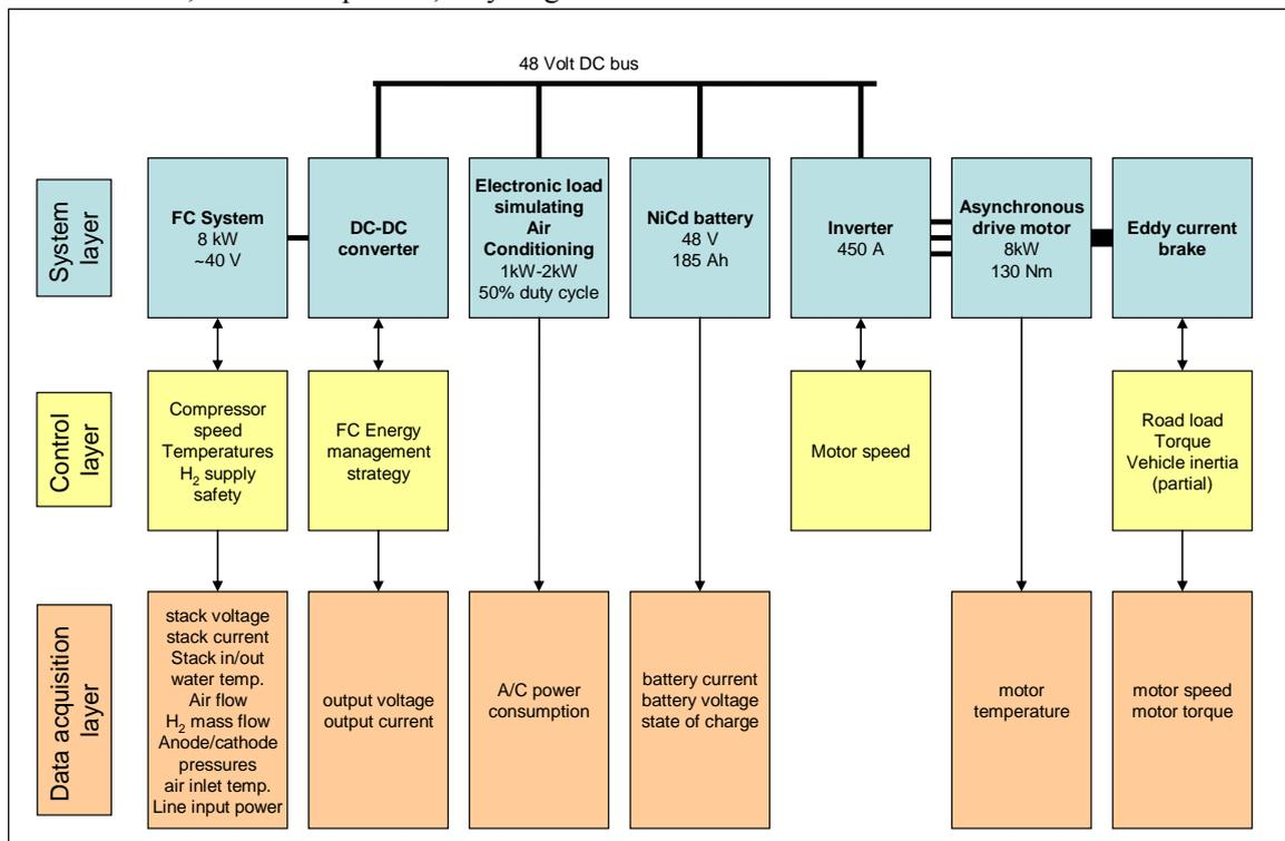
Figure 2. Schematic overview of the HAN fuel cell hybrid drive train test facility.
