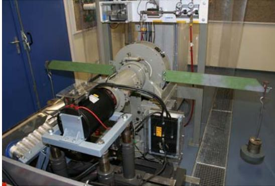
Figure 1. Impression of the Fuel cell hybrid drive train test facility, showing the drive motor, motor inverter and eddy current brake with torque sensor calibration arms attached. In the background, the cabinet with fuel cell stack can be seen.
