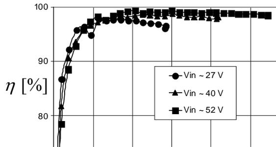
Figure 9. Typical efficiency vs. output power data for the DC-DC converter at different input voltage levels. Output voltage: 75 [V].
