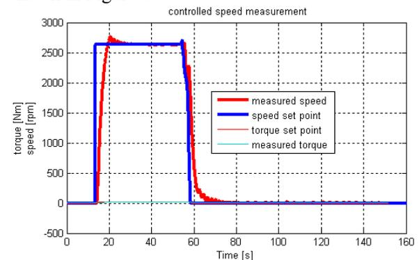
Figure 6. Closed loop step response of the speed control loop at a torque of 15 Nm
