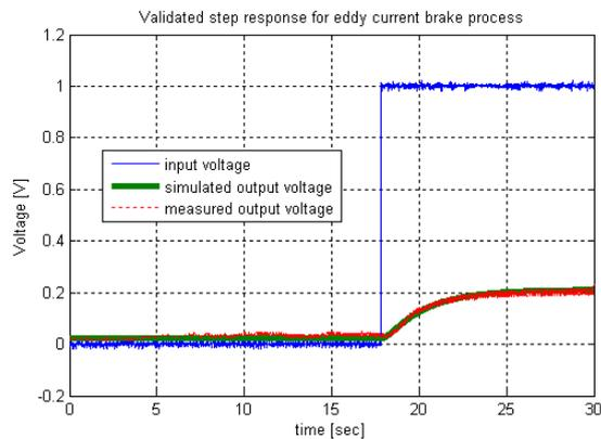
Figure 4. Open loop step response of eddy current brake
