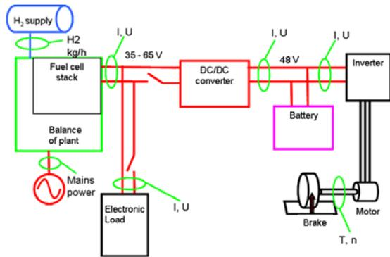
Figure 3. Physical test rig layout, showing power flow measurement points.
