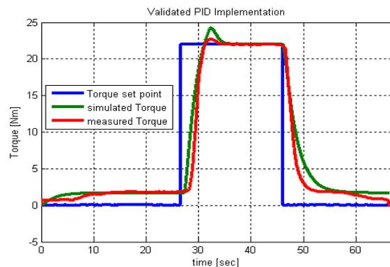
Figure 5. Closed loop response at 800 [rpm] motor speed.
